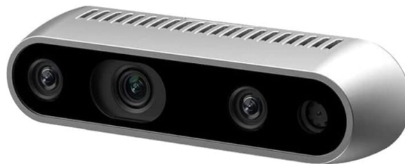
Fig. 3.10 The Intel RealSense D435 Camera. It is a 3D depth camera that uses advanced stereo vision technology to capture depth information and enable applications such as augmented reality, virtual reality, and 3D scanning. It features a depth sensor with a range of up to 10 meters, an RGB sensor with a resolution of 1920x1080 at 30fps, and an infrared sensor for improved depth perception in low-light conditions.
